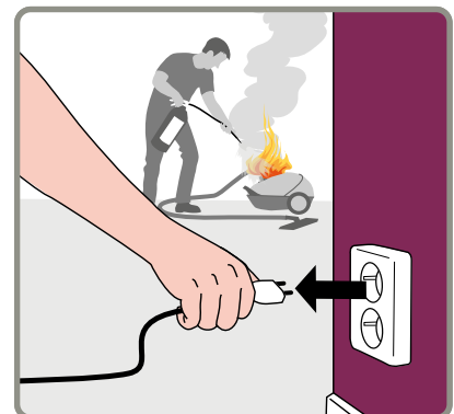
Electrical appliances on fire: First, unplug the appliance. Smother the fire with a fire blanket or water. With a powder extinguisher, you can extinguish the fire immediately, without unplugging the appliance.
