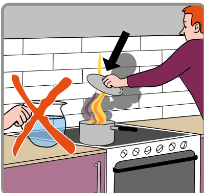
Fire in a saucepan or frying pan: Use the lid or a fire blanket to smother the fire. Never use water. Water causes the flames to spread.
